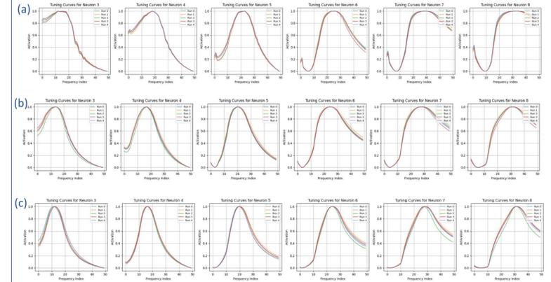
(a-c) Normalized tuning curves of a subset of neurons across 5 runs demonstrate robustness, frequency selectivity and sideband inhibition at (a) 4 ms, (b) 16 ms, and (c) 64 ms timescales.
