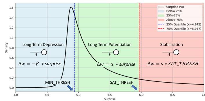
Surprise distribution estimated from MelNet is used to set thresholds at quartiles (MIN\_THRESH, SAT\_THRESH), driving a three-factor learning rule: depression ( $\beta$ ) for low surprise, potentiation ( $\alpha$ ) for moderate surprise, and stabilization ( $\gamma$ ) for high surprise. Post-update, sparsity is enforced via L1-norm gradient descent on activations.
